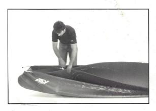
Place foam mat inside with the black side up at bottom of canoe skin by folding mat in half lengthwise and holding edges together. Foam mat must be centered sideways and lie as high in the bow as in the stern.
