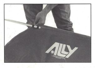
Lay canoe skin flat on its side with edges together and even. Slide gunwales (E) into channel at edge of skin.
